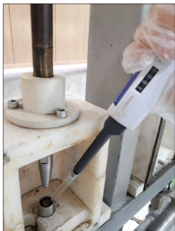
Figure 1: Microbial solution recharge during cyclic load
